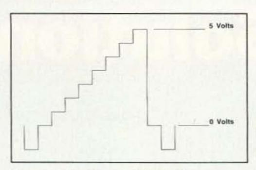
Figure 2. Waveform at TP-3 with gray-scale input.
